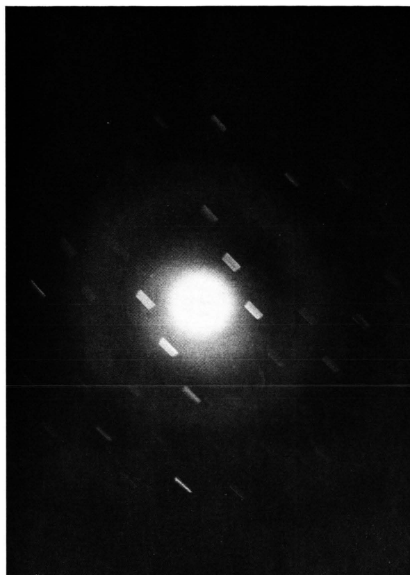
Fig. 3. Low-magnification multiple images from which the relative orientation of crystal edges and axes can be determined.
